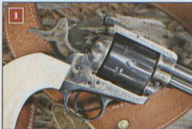
1) The hammer of The Last Frontier is color cased to match the beautiful colors on the Colt's frame. 2) The detail of the custom .45 Colt cylinder is seen with its beveled front and correctly sized flutes just like turn of the century Colts. 3) All exterior screws on The Last Frontier are fire-blued for that extra touch.
