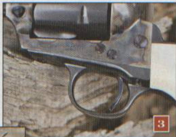
1) The hammer of The Last Frontier is color cased to match the beautiful colors on the Colt's frame. 2) The detail of the custom .45 Colt cylinder is seen with its beveled front and correctly sized flutes just like turn of the century Colts. 3) All exterior screws on The Last Frontier are fire-blued for that extra touch.
