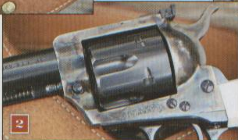
1) The hammer of The Last Frontier is color cased to match the beautiful colors on the Colt's frame. 2) The detail of the custom .45 Colt cylinder is seen with its beveled front and correctly sized flutes just like turn of the century Colts. 3) All exterior screws on The Last Frontier are fire-blued for that extra touch.
