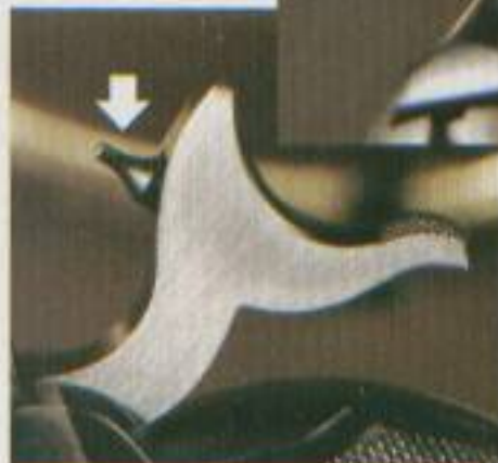
Current guns still retain the classic fixed firing pin in the hammer.
