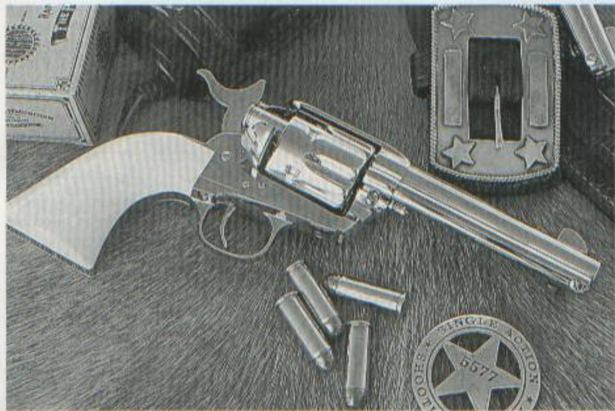
With custom cylinder flutes and period radiusing, Peacemaker Specialists' matching Colts are tastefully dehorned on their exterior.
