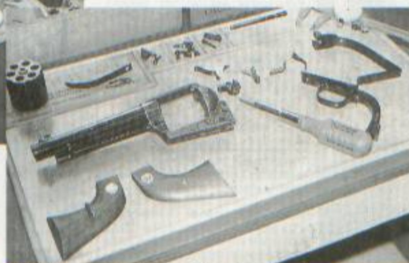
Pistol disassembly is required so all parts and surfaces can be examined, polished, refitted, or replaced as needed.
