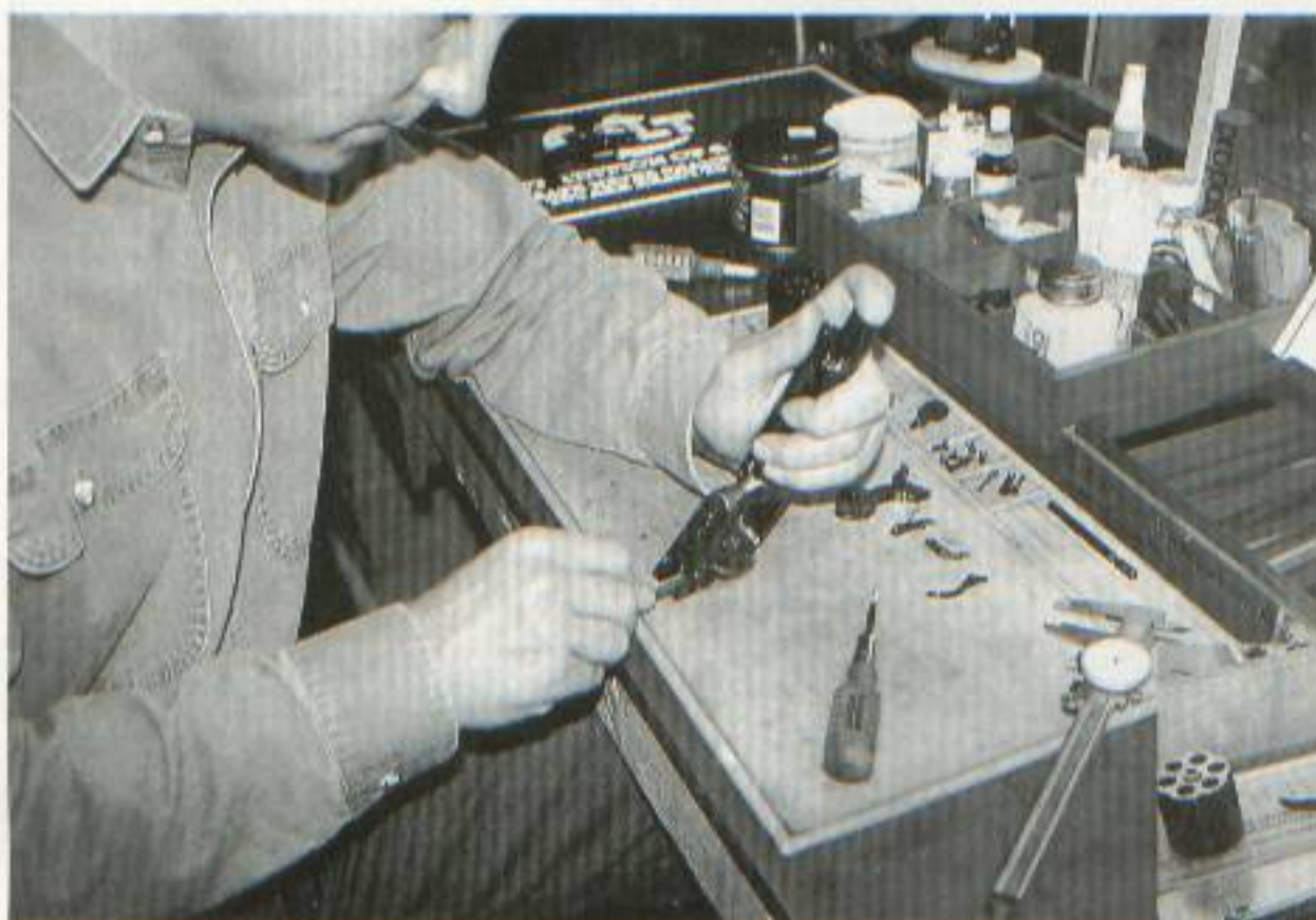
Eddie Janis stones the internal surfaces of a Colt frame during an action job.
