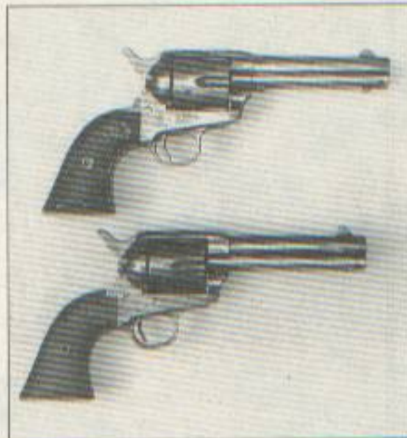
An early black-powder frame SAA (top), which used a screw to hold the cylinder base pin, and a post-1896 "smokeless" frame (bottom), which features a spring-loaded cross pin.
